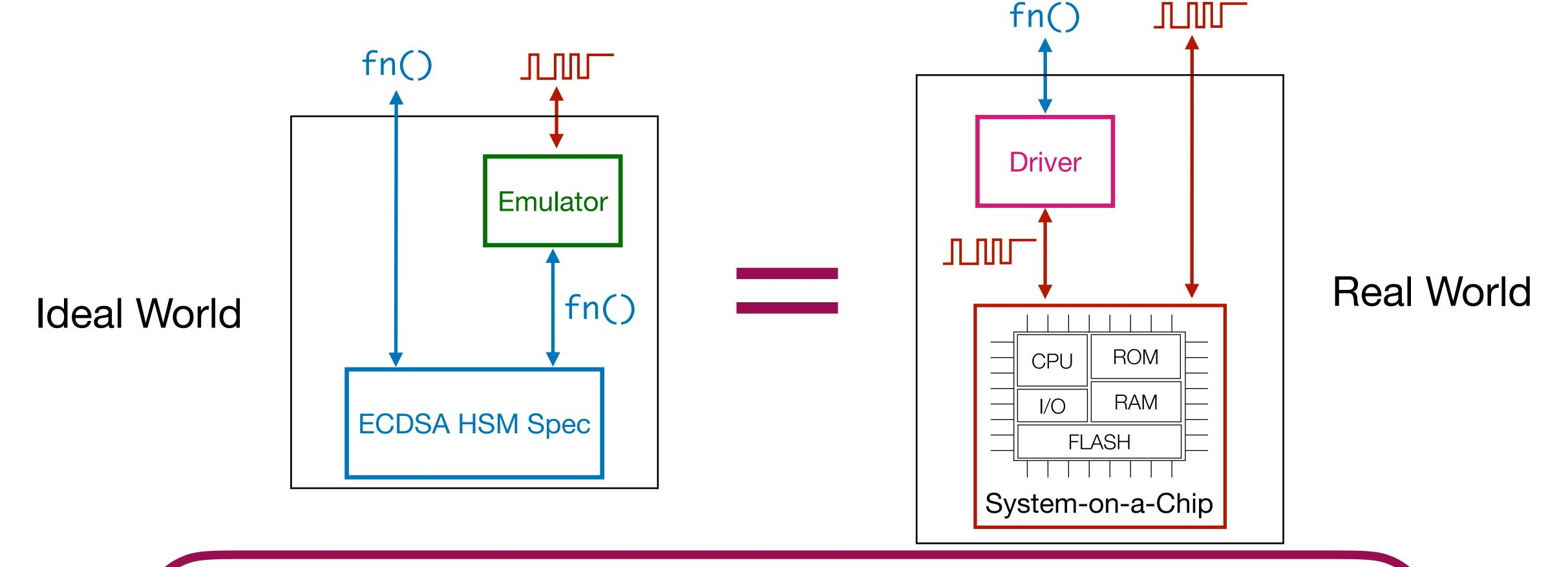
Circuit implements spec, and it doesn't leak any additional information through its cycle-precise wire-level behavior
